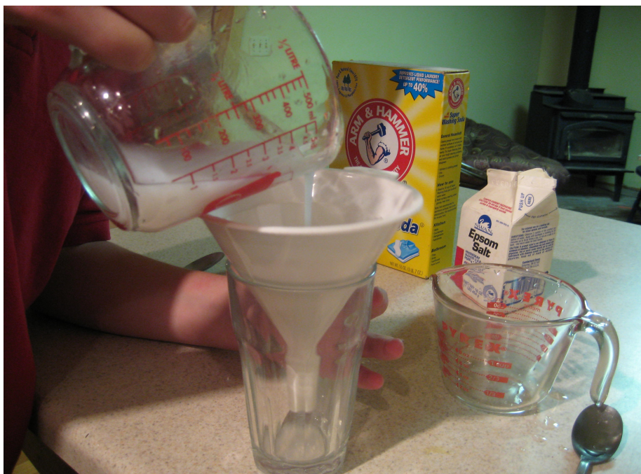
Pour the solution slowly through the funnel filter so that the solution never goes over the top edge of the filter paper.
